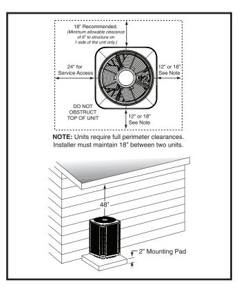
**Figure 1. Clearance Requirements**
