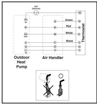
Figure 4. Typical Thermostat Connections
