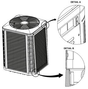
Figure 6. Panel Installation
