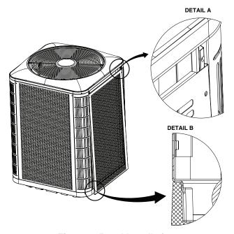
Figure 3. Panel Installation
