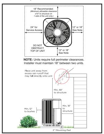
Figure 1. Clearance Requirements
