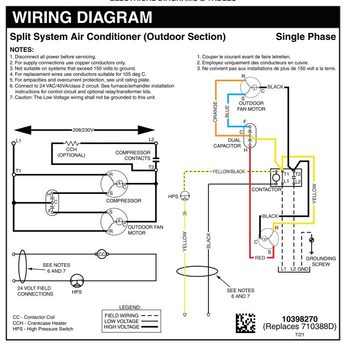
Figure 5. Wiring Diagram for \*SA3BD4M (1.5 - 4 Ton Units)
