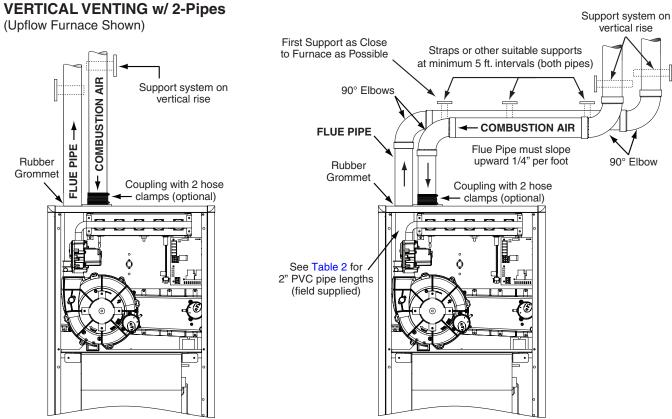
Figure 35. Horizontal & Vertical Venting
