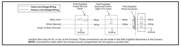
Figure 24. Line Voltage Field Wiring
