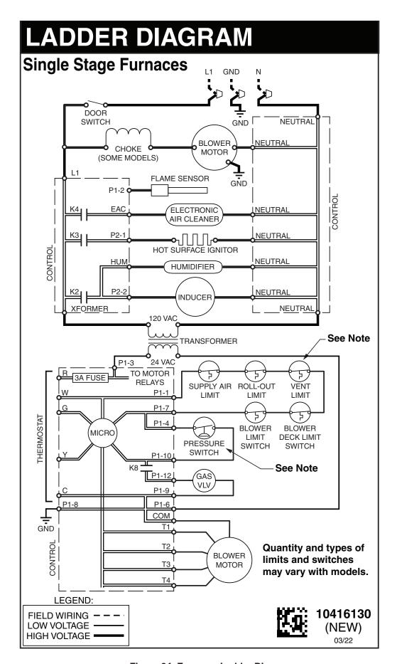
Figure 34. Emerson Ladder Diagram
