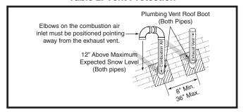
**Figure 10. Vertical Vent Termination**
