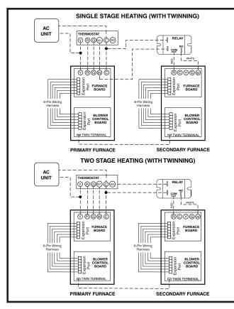
Figure 27. Nordyne/UTEC Single & Two Stage Twinning
