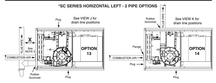
Figure 38. Venting Options for 2-Pipe Horizontal Installations (\*SC Series)
