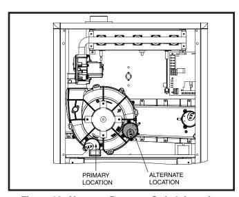
Figure 16. Alternate Pressure Switch Location
