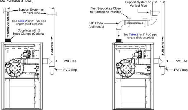
Figure 39. Horizontal & Vertical Venting
