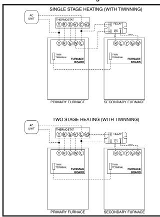
Figure 28. Emerson Single & Two Stage Twinning
