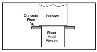
Figure 13. Furnace on a Concrete Slab
