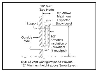
Figure 9. Alternate Horizontal Vent Installation
