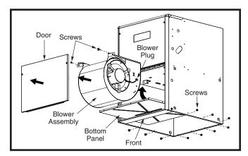
Figure 21. Bottom Panel Removal
