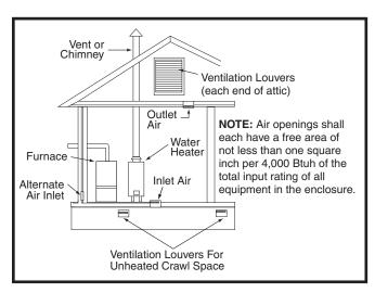
Figure 4. Combustion Air Drawn from a Crawl Space or Vented Attic
