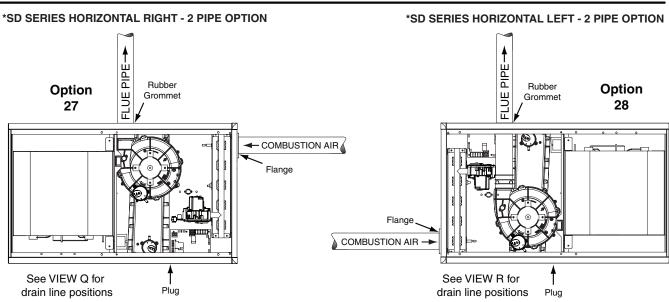
Figure 41. Venting Options for Horizontal Installations (\*SD Series)
