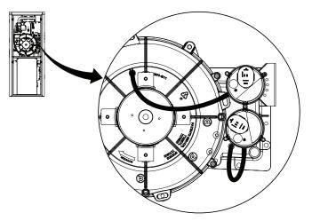
Figure 14. Pressure Switch Tubing for \*SC038 Furnaces Only
