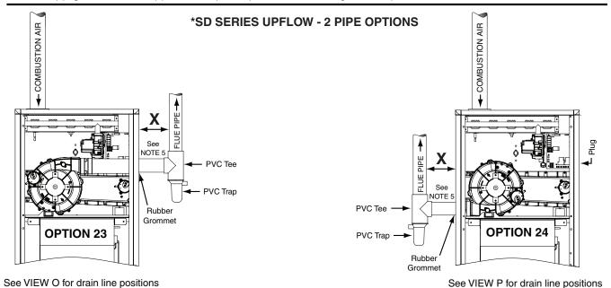
Figure 40. Venting Options for Upflow Installations (\*SD Series)
