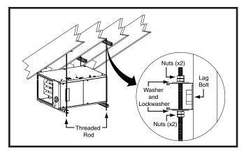
Figure 12. \*SC & \*SD Horizontally Suspended in an Attic
