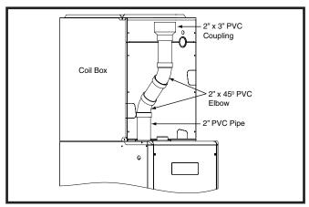
Figure 20. Optional PVC Pipe Installation
