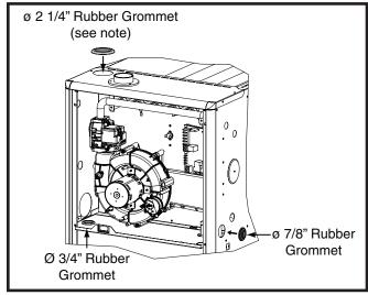
Figure 18. Rubber Grommets
