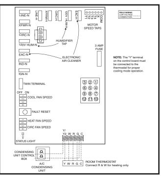
Figure 26. Emerson Low Voltage Field, Fourwire Heating/Cooling Applications
