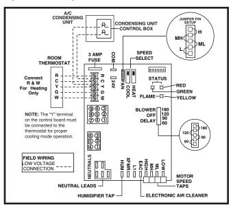
Figure 25. Nordyne/UTEC Low Voltage Field, Fourwire Heating/Cooling Applications
