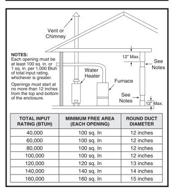
Figure 2. Combustion Air Drawn from Inside
