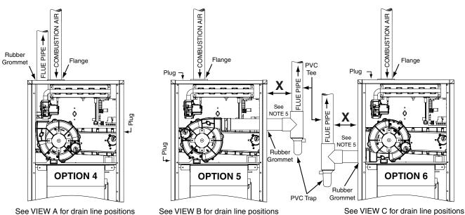
Figure 36. Venting Options for Upflow Installations (\*SC Series)
