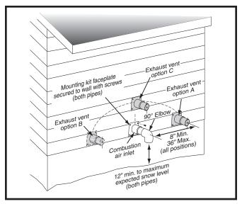
Figure 7. Inlet & Exhaust Pipe Clearances
