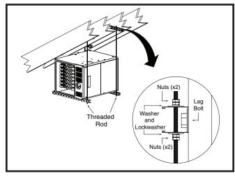
Figure 8. \*SA Horizontally Suspended in Attic
