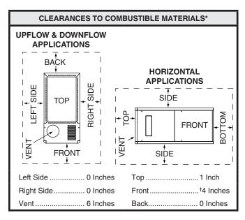
$^{\dagger}\text{Allow}\,24\,\text{in}$  . minimum clearance for servicing. Recommended clearance is 36 in.
