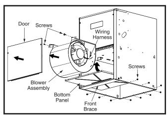
Figure 11. Bottom Panel Removal
