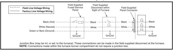
Figure 14. Line Voltage Field Wiring
