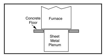
Figure 9. Furnace on a Concrete Slab
