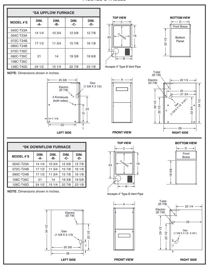
Figure 20. Furnace Dimensions
