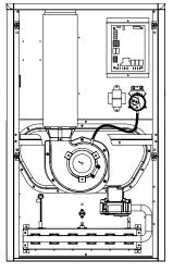
Figure 10. Pressure Switch Tubing for \*SA & \*SK Furnaces
