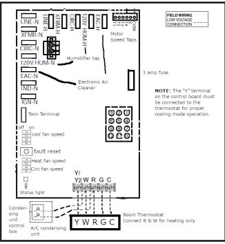
Figure 16. Emerson Low Voltage Field, Fourwire Heating/Cooling Applications
