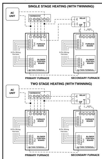
Figure 17. Nordyne/UTEC Single Stage Twinning
