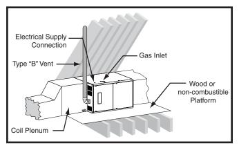
Figure 7. \*SA Horizontal Installed on a Platform
