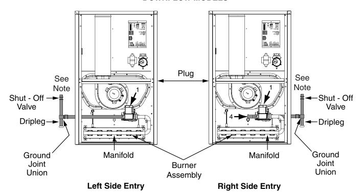
NOTE: Some utilities require Shut- Off Valve to be 4 - 5 feet above floor.
