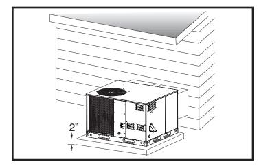
Figure 4. Ground Level Installation
