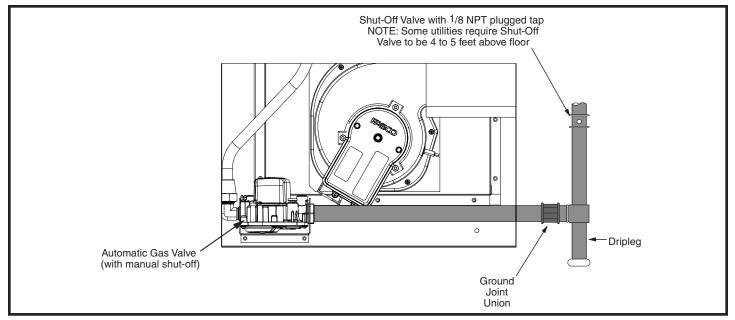
Figure 7. Typical Gas Hookup - Right Side Entry
