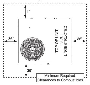
Figure 1. Clearance Requirements
