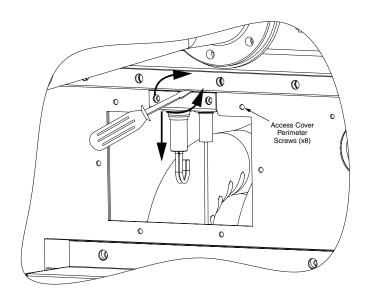
Figure 9. Ignitor Flame Sensor Bracket
