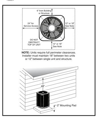
Figure 1. Clearance Requirements
