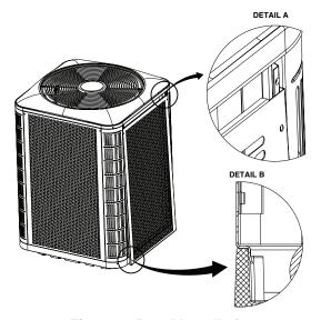
Figure 4. Panel Installation
