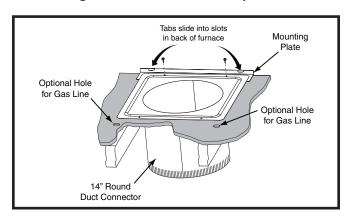
Figure 15. Round Duct Connector
