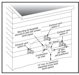
Figure 1. Inlet & Exhaust Pipe Clearances
