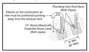
**Figure 4. Vertical Vent Termination**
