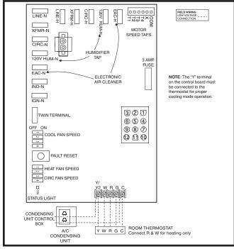
Figure 23. Emerson Low Voltage Field, Fourwire Heating/Cooling Applications
