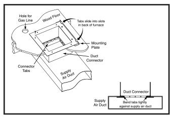
Figure 11. Finger Tabbed Duct Connector
