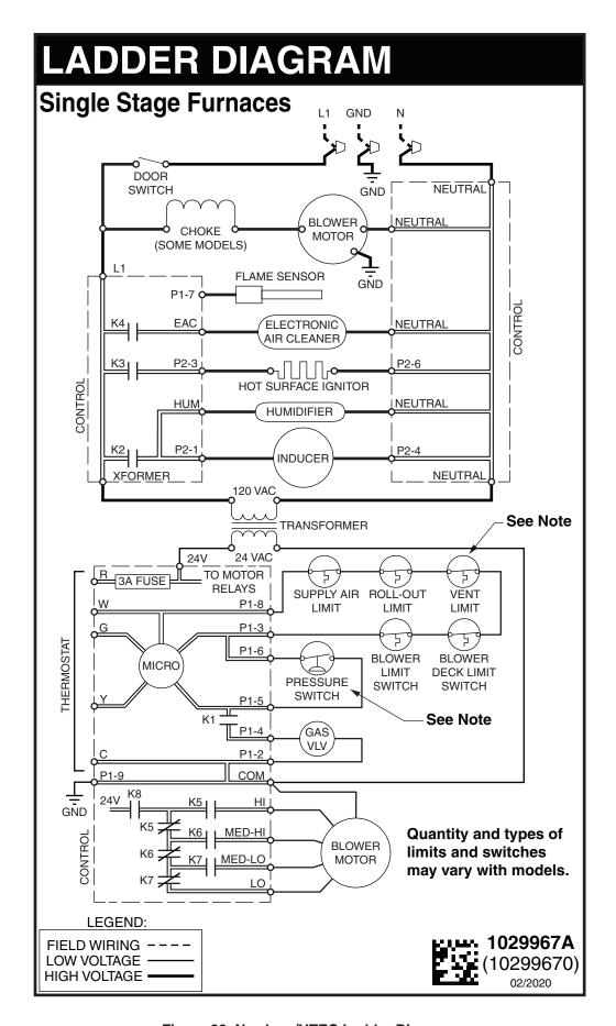
Figure 32. Nordyne/UTEC Ladder Diagram
