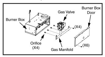
Figure 20. Orifice Removal
