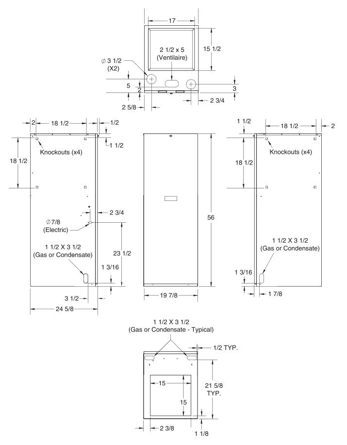
Figure 27. Top Return Cabinets (Without Coil Box)
