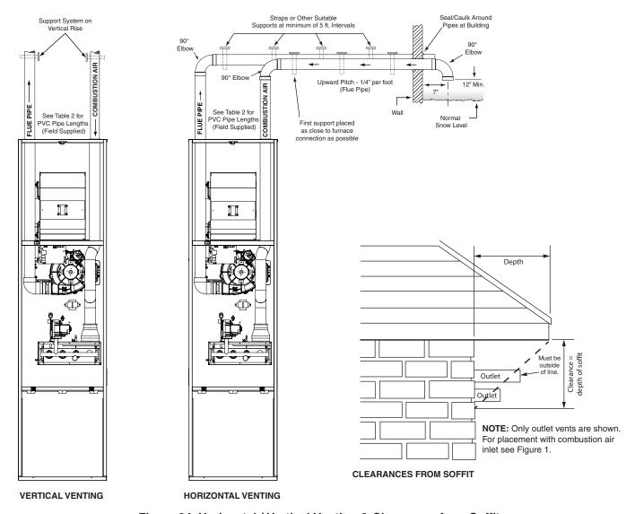
Figure 34. Horizontal / Vertical Venting & Clearances from Soffit
