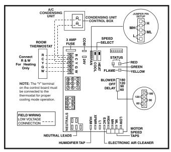
Figure 22. Nordyne/UTEC Low Voltage Field, Fourwire Heating/Cooling Applications
