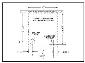
Figure 10. Ceiling Cut-Out Dimensions
