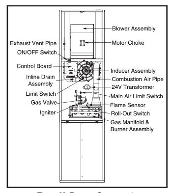
Figure 23. Furnace Components
