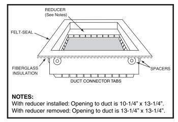
Figure 8. Duct Connector
