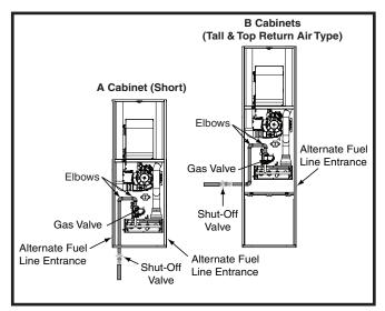
Figure 18. Typical Gas Connections
