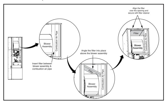
Figure 7. Filter Installation
