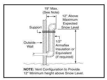
Figure 3. Alternate Horizontal Vent Installation
