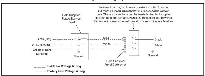
Figure 21. Line Voltage Field Wiring
