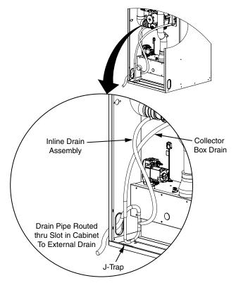
Figure 17. Condensate Drainage
