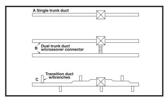
Figure 6. Typical Supply Duct Systems
