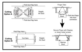
Figure 12. Screw-Down Duct Connector
