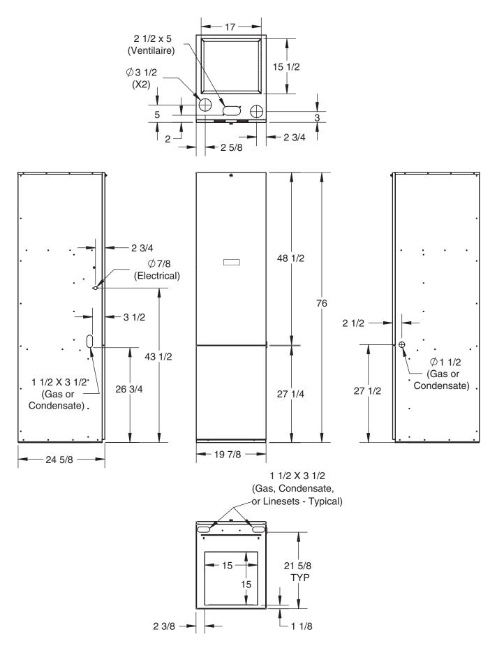
Figure 29. Top Return Cabinets (With Coil Box) (return cabinets ending in 'ACM)
