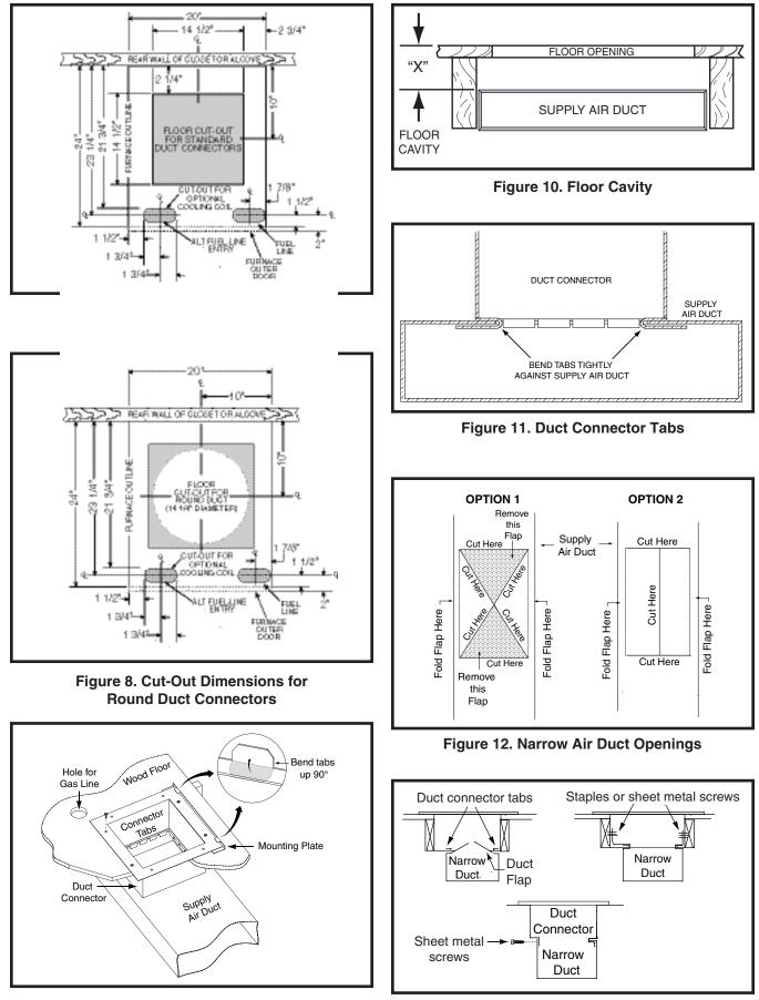
Figure 9. Standard Duct Connector Installed
