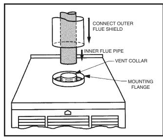
Figure 23. Combustion Air Pipe Connection
