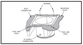
Figure 14. Round Duct Connector Installed
