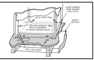
Figure 16. "A" Cabinet Furnace on Coil Cabinet
