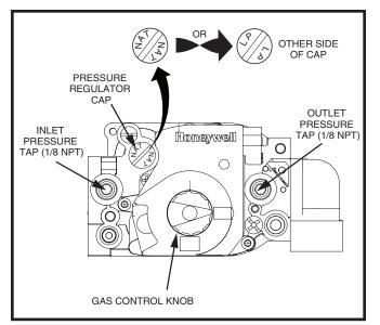
Figure 29. Honeywell/Resideo Gas Valve
