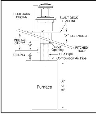
Figure 17. Ceiling Cavity Depth
