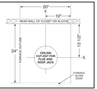
Figure 20. Cut-Out Dimensions for Flue & Roof Jack
