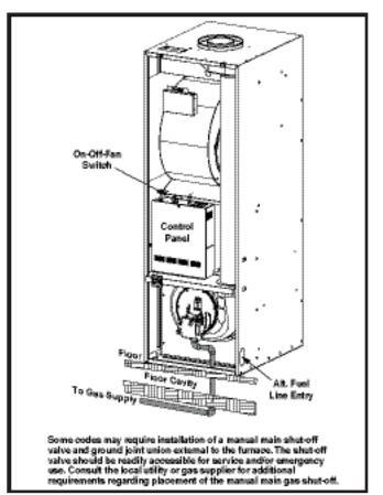
Figure 28. Typical Gas Piping
