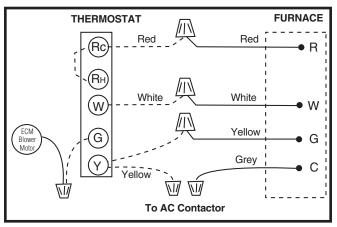
Figure 26. Thermostat Wiring for UTEC/NORDYNE Control boards
