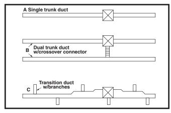
Figure 6. Typical Supply Duct System
