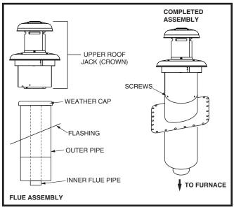
Figure 24. Roof Jack Crown
