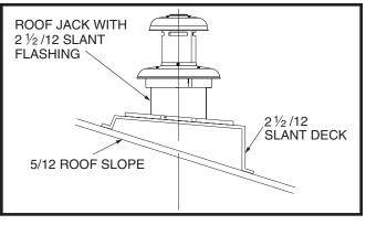
Figure 19. Example of 2½ / 12 Slant Jack with Flashing
