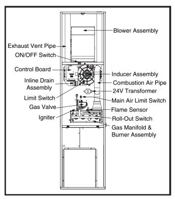
Figure 24. Furnace Components
