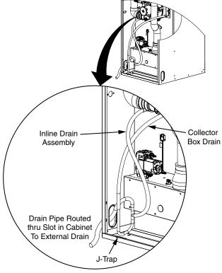
Figure 18. Condensate Drainage
