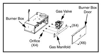
Figure 21. Orifice Removal
