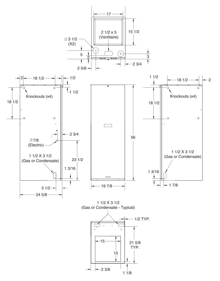
Figure 28. Top Return Cabinets (Without Coil Box)
