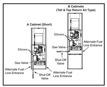
Figure 19. Typical Gas Connections
