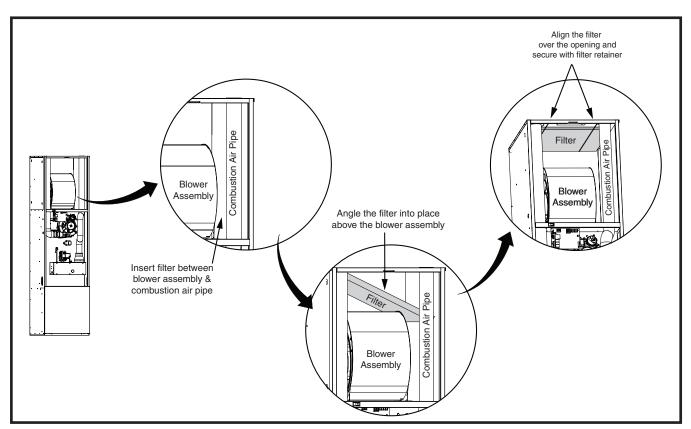
Figure 8. Filter Installation
