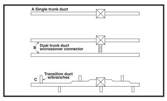
Figure 7. Typical Supply Duct Systems
