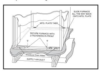
Figure 17. Cabinet Furnace on Supply Air Duct
