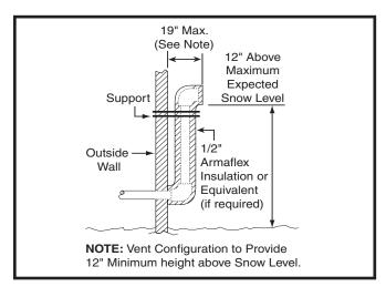
Figure 3. Alternate Horizontal Vent Installation
