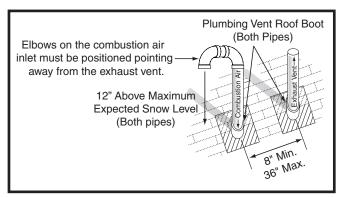
**Figure 4. Vertical Vent Termination**
