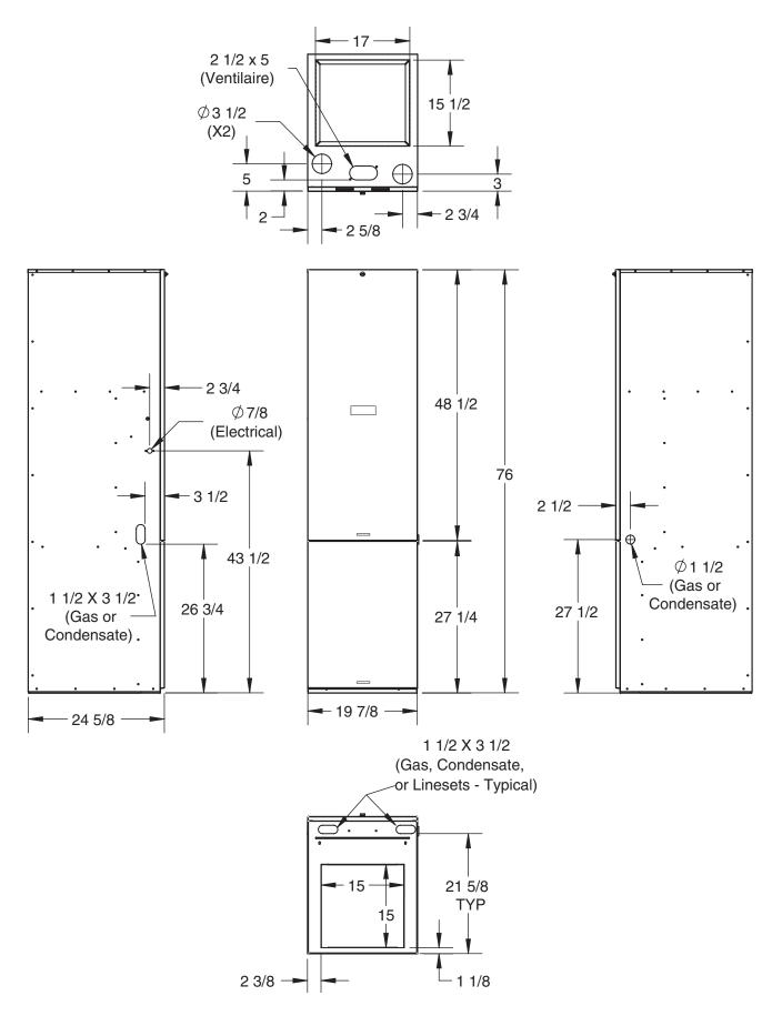
Figure 30. Top Return Cabinets (With Coil Box) (return cabinets ending in 'ACM)
