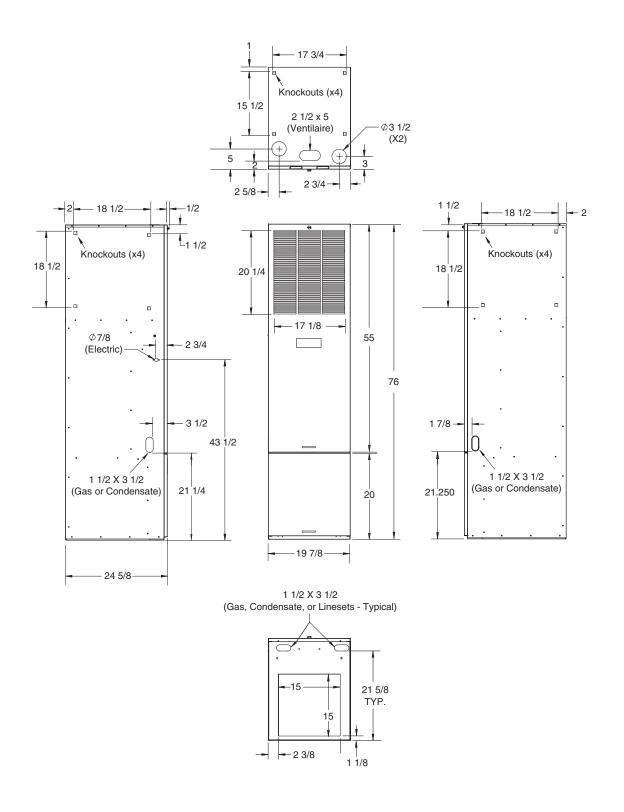
Figure 26. Front Return Cabinets (With Coil Box) (return cabinets ending in 'ABM)
