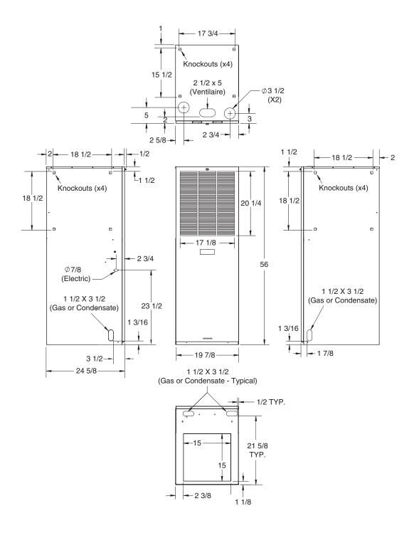
Figure 25. Front Return Cabinets (Without Coil Box)
