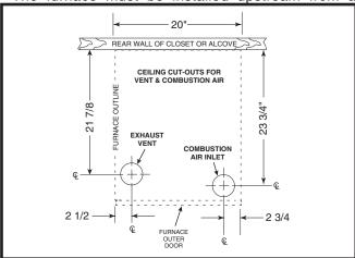
Figure 11. Ceiling Cut-Out Dimensions
