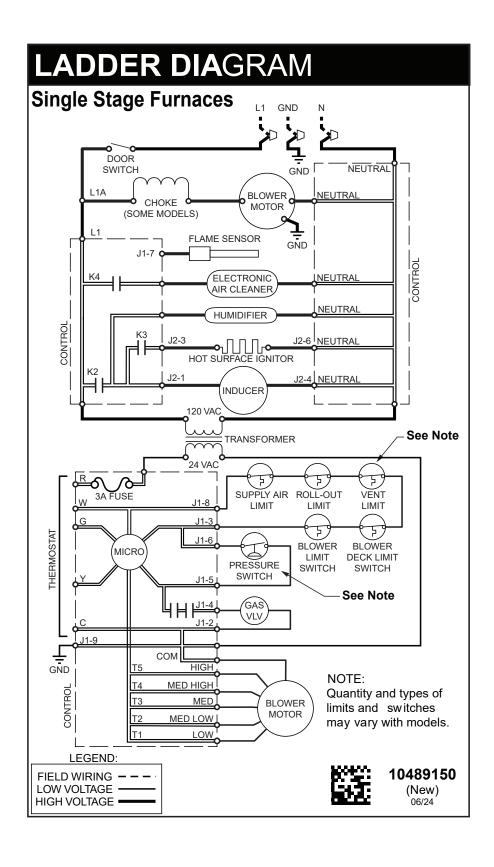
Figure 32. Nordyne Channel Ladder Diagram
