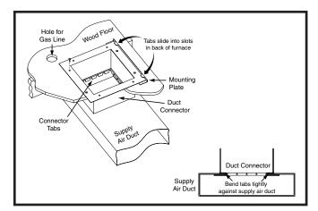
Figure 12. Finger Tabbed Duct Connector
