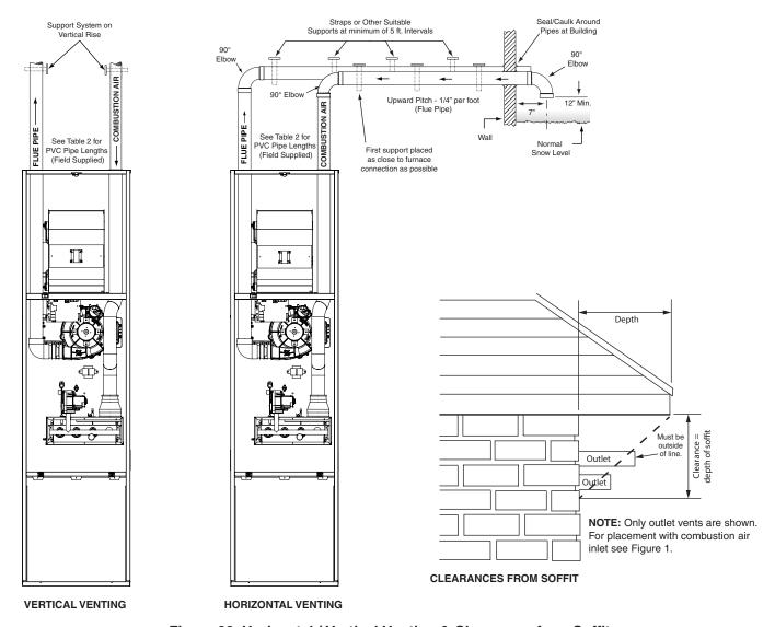
Figure 33. Horizontal / Vertical Venting & Clearances from Soffit
