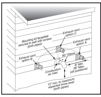
Figure 1. Inlet & Exhaust Pipe Clearances
