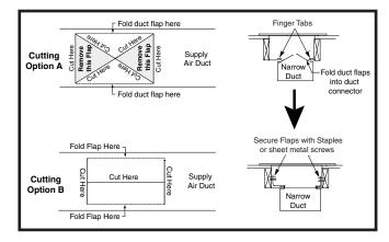
Figure 13. Screw-Down Duct Connector
