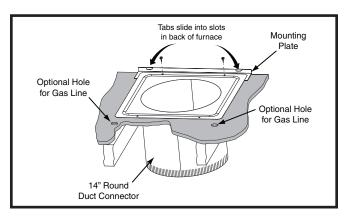
Figure 16. Round Duct Connector
