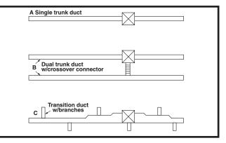
Figure 7. Typical Supply Duct Systems
