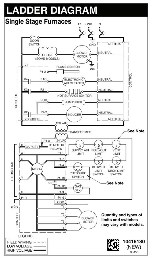
Figure 35. Emerson Ladder Diagram
