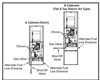
Figure 19. Typical Gas Connections
