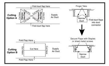
Figure 13. Screw-Down Duct Connector
