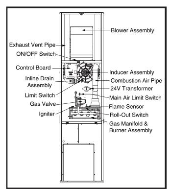
Figure 25. Furnace Components
