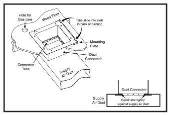
Figure 12. Finger Tabbed Duct Connector
