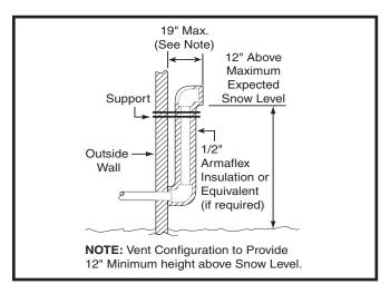
Figure 3. Alternate Horizontal Vent Installation
