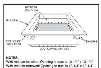
Figure 9. Duct Connector
