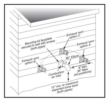
Figure 1. Inlet & Exhaust Pipe Clearances
