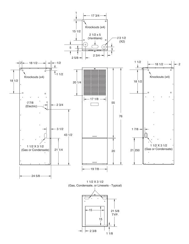
Figure 27. Front Return Cabinets (With Coil Box) (return cabinets ending in 'ABM)
