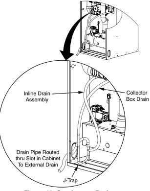
Figure 18. Condensate Drainage
