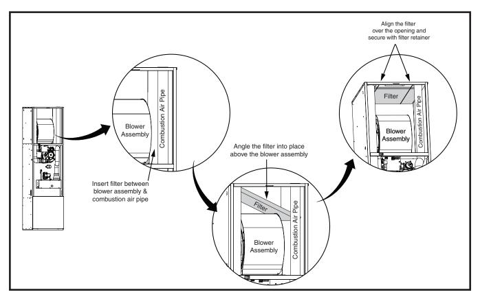
Figure 8. Filter Installation
