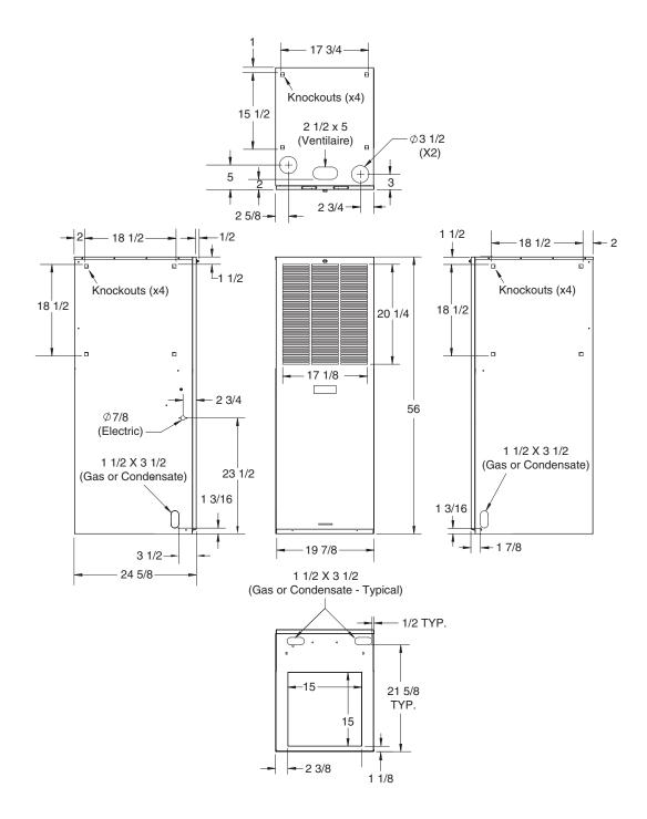
Figure 26. Front Return Cabinets (Without Coil Box)
