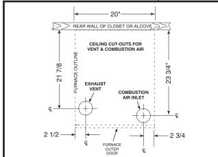
Figure 11. Ceiling Cut-Out Dimensions
