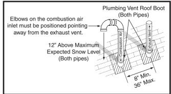
**Figure 4. Vertical Vent Termination**
