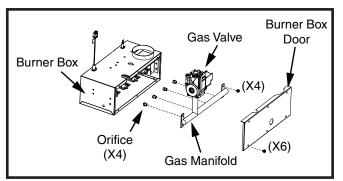
Figure 21. Orifice Removal
