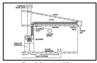
Figure 5. General Install Setup
