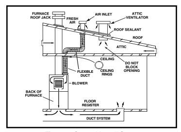
Figure 6. General Install Setup
