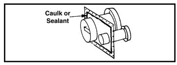
Figure 9. Sealant Application
