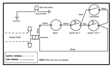
Figure 7. VentilAire™ IV Wiring Diagram
