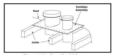
Figure 4. Ventilator Roof Alignment
