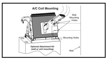
Figure 2. Downflow Electric Furnace with A/C
