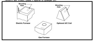
Figure 1. Plastic Inlet Fitting Location
