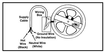
Figure 8. Wire Connections
