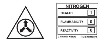
C84DA coils are pressurized with Nitrogen at the factory. Avoid direct face exposure or contact with valve when gas is escaping. Always ensure adequate ventilation is present during the depressurization process. Any uncertainties should be addressed before proceeding.
