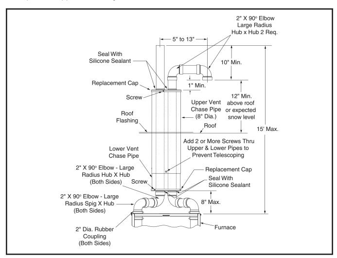
Figure 1. Vent & Combustion Air Intake Pipe Installation
