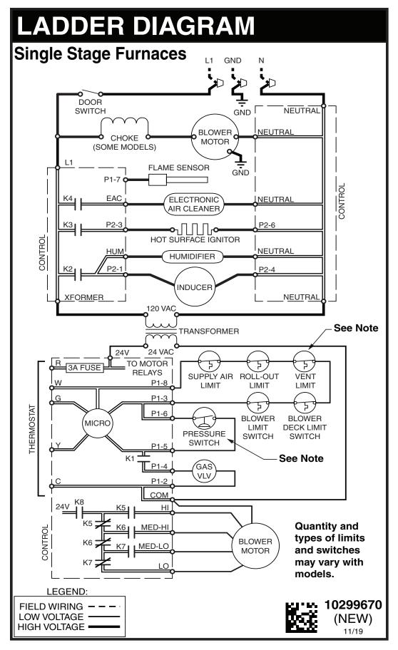
Figure 46. MG3P Ladder Diagram
