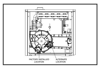
Figure 26. Alternate Pressure Switch Location
