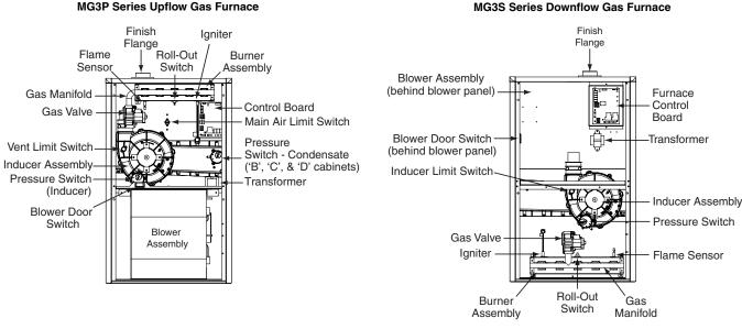
Figure 55. MG3(P,S) Component Locations
