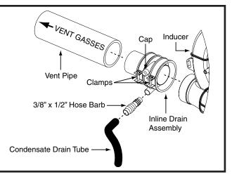
Figure 29. Inline Drain Assembly
