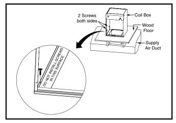
Figure 20. A/C Coil Box Installation
