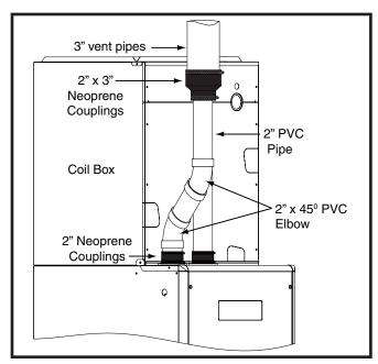
Figure 34. Alternate vent Pipe Installation
