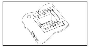
Figure 15. Duct Connector Side Plates
