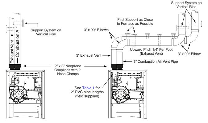
Figure 51. MG3P Horizontal & Vertical Venting
