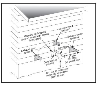
Figure 7. Inlet & Exhaust Pipe Clearances
