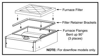
Figure 32. Filter Retainer Brackets
