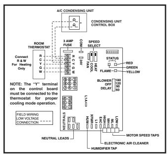
Figure 42. Low Voltage Field, Four-wire Heating / Cooling Applications
