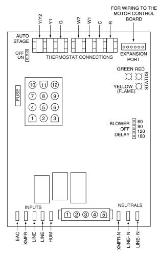
Figure 50. Two-Stage Furnace Control Board
