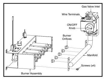
Figure 37. Burner & Manifold Assembly
