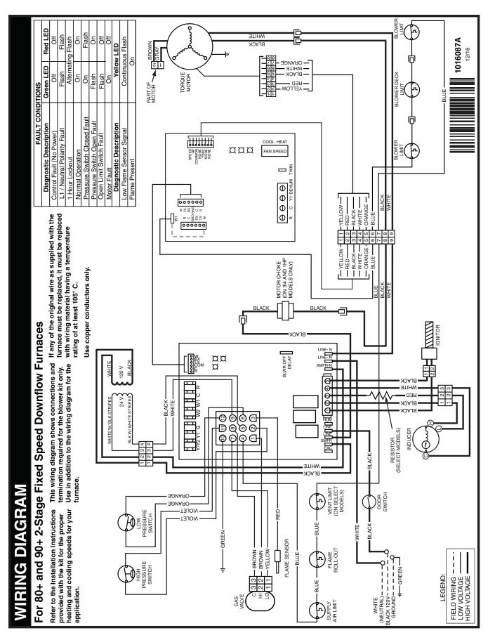
Figure 47. MG3S Wiring Diagram
