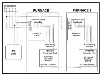
Figure 43. Single Stage Twinning
