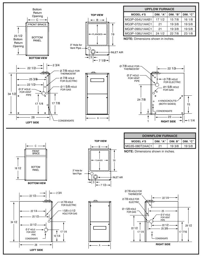
Figure 44. Furnace Dimensions
