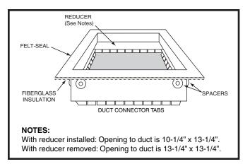
Figure 12. Duct Connector
