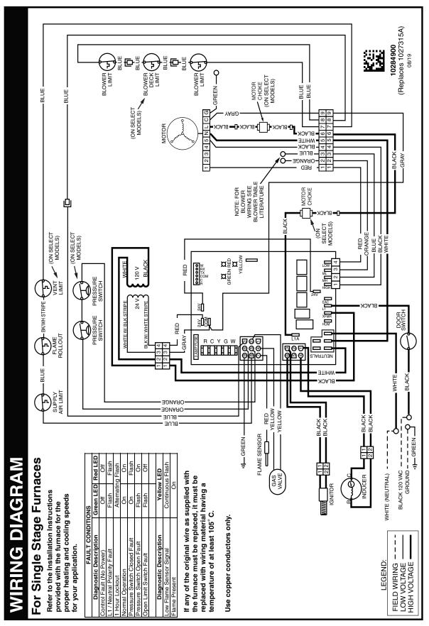
Figure 45. MG3P Wiring Diagram
