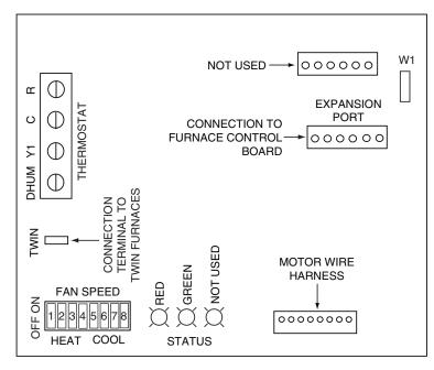
Figure 49. Two-Stage Fixed Speed Motor Control Board
