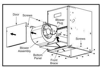
Figure 22. Bottom Panel Removal
