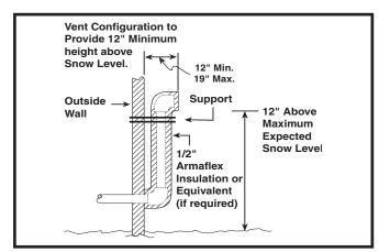
Figure 9. Alternate Horizontal Vent Installation
