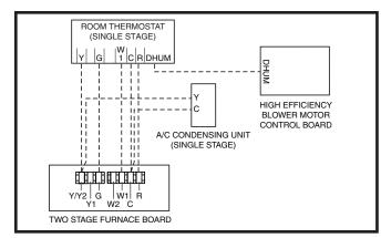
Figure 38. Wiring Configuration 1
