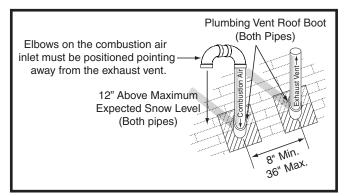
Figure 10. Vertical Vent Termination
