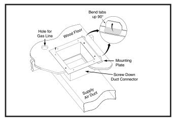
Figure 18. Screw-Down Duct Connector
