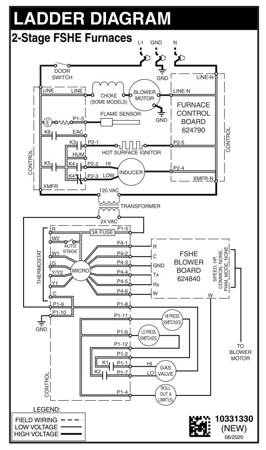
Figure 48. MG3S Ladder Diagram
