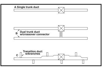
Figure 11. Typical Supply Duct System
