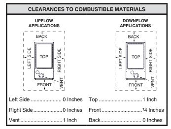
$^{\dagger}\text{Allow}\,24\,\text{in.}$  minimum clearance for servicing. Recommended clearance is 36 in.
