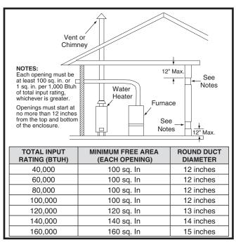
Figure 2. Combustion Air Drawn from Inside
