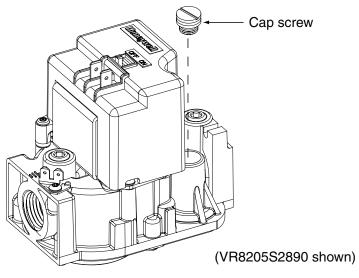
Figure 2. Cap Screw Removal
