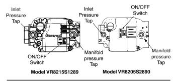
2-STAGE VALVE ON/OFF Knob Inlet Pressure Tap
