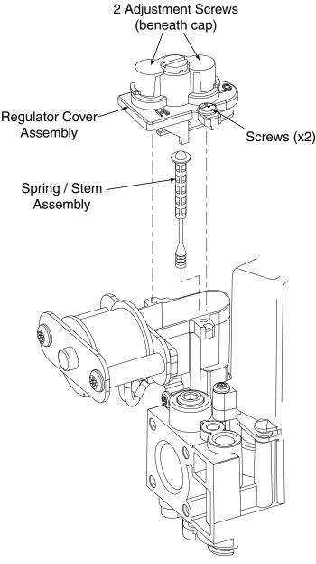
Figure 4. Spring / Stem Assembly Removal
