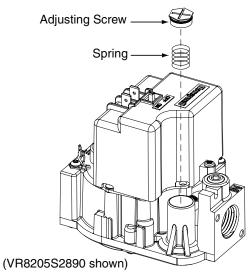
Figure 3. Pressure Regulator Spring & Adjustment Screw Removal
