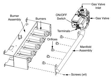
Figure 1. Typical Burner & Manifold Assembly
