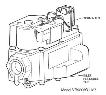
Fig. 8. Gas conversion kit: inlet
