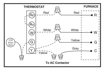
Figure 25. Thermostat Wiring for UTEC/NORDYNE Control boards
