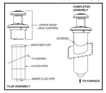
Figure 23. Roof Jack Crown
