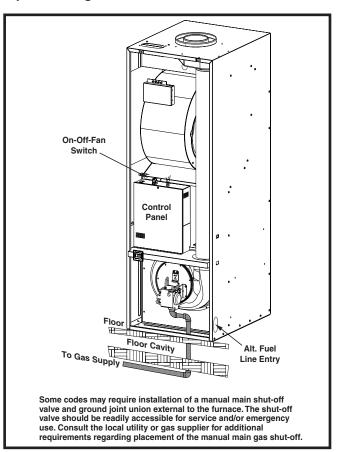
Figure 27. Typical Gas Piping
