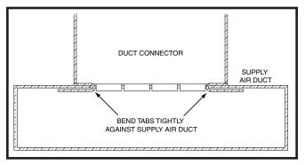
Figure 10. Duct Connector Tabs
