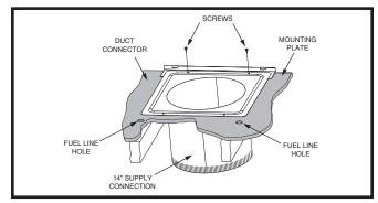
Figure 13. Round Duct Connector Installed
