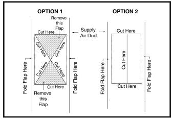
Figure 11. Narrow Air Duct Openings
