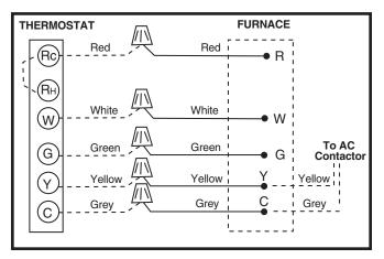
Figure 26. Thermostat Wiring for Emerson/ Copeland control boards
