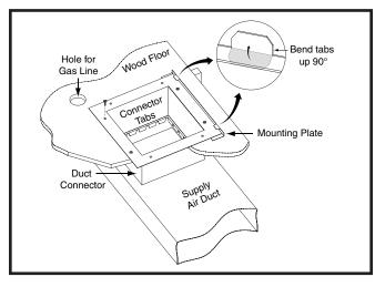
**Figure 8. Standard Duct Connector Installed**
