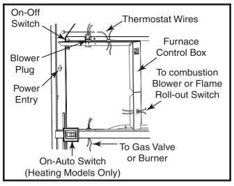
Figure 24. Control Panel (All Models)
