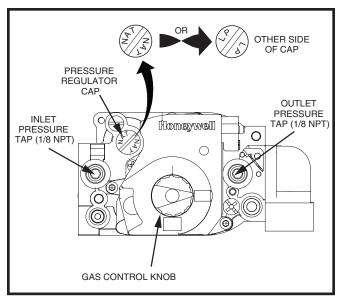
Figure 28. Honeywell/Resideo Gas Valve
