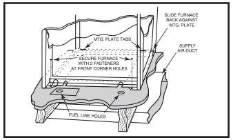
Figure 15. "A" Cabinet Furnace on Coil Cabinet
