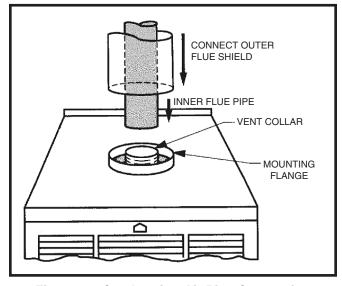
Figure 22. Combustion Air Pipe Connection
