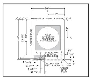
Figure 7. Cut-Out Dimensions for Round Duct Connectors
