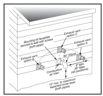
Figure 1. Inlet & Exhaust Pipe Clearances
