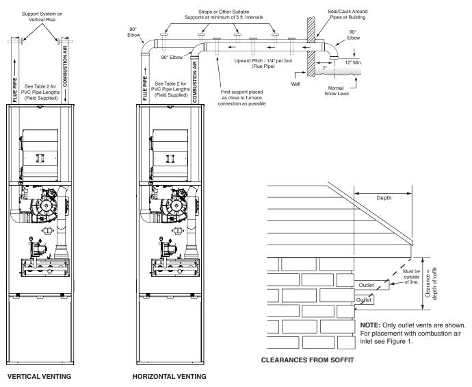
Figure 32. Horizontal / Vertical Venting & Clearances from Soffit
