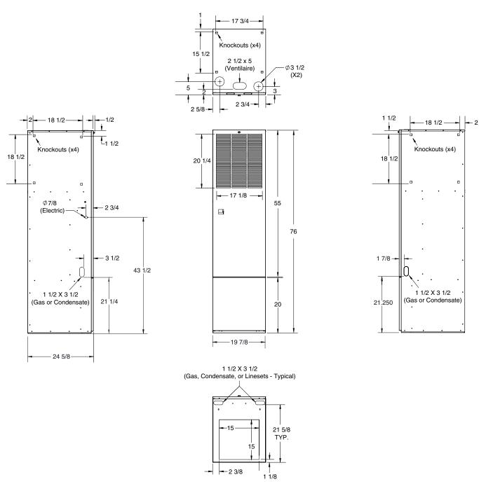
Figure 25. Front Return Cabinets (With Coil Box)
