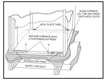
Figure 16. Cabinet Furnace on Supply Air Duct
