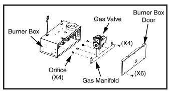
Figure 20. Orifice Removal
