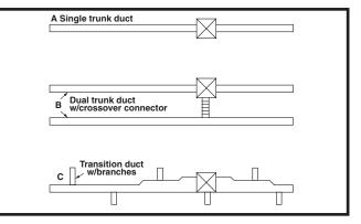
Figure 6. Typical Supply Duct Systems
