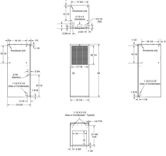
Figure 24. Front Return Cabinets (Without Coil Box)
