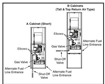
Figure 18. Typical Gas Connections
