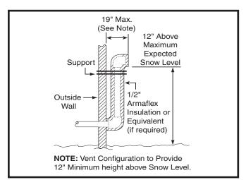
Figure 3. Alternate Horizontal Vent Installation
