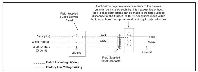
Figure 21. Line Voltage Field Wiring
