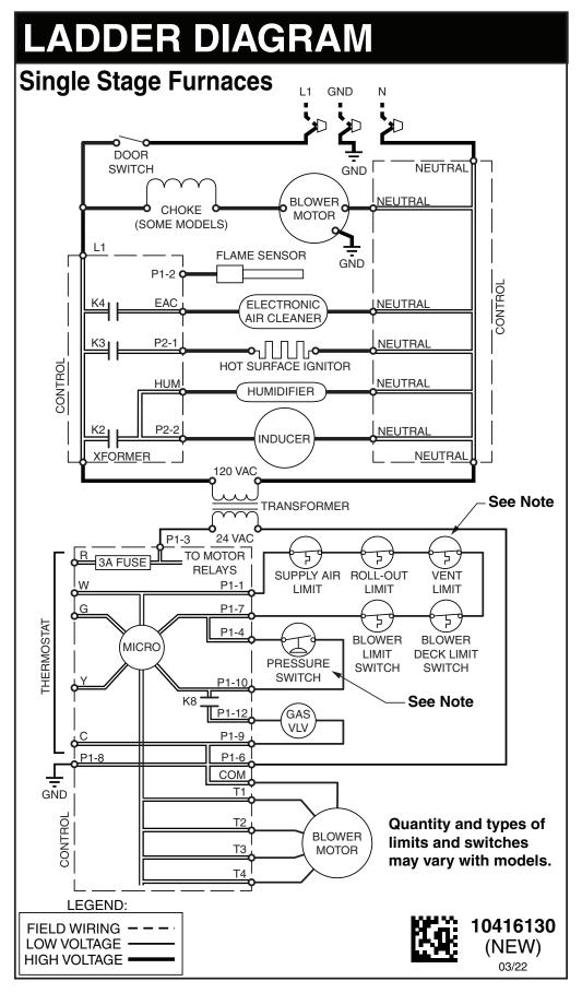
Figure 31. Emerson Ladder Diagram
