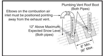
**Figure 4. Vertical Vent Termination**
