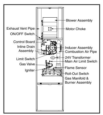
Figure 23. Furnace Components
