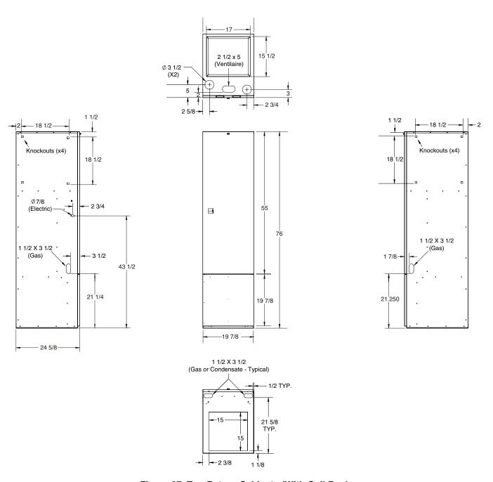
Figure 27. Top Return Cabinets (With Coil Box)
