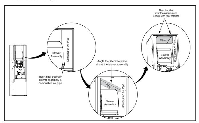
Figure 7. Filter Installation
