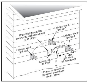
Figure 1. Inlet & Exhaust Pipe Clearances
