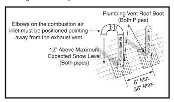
**Figure 4. Vertical Vent Termination**
