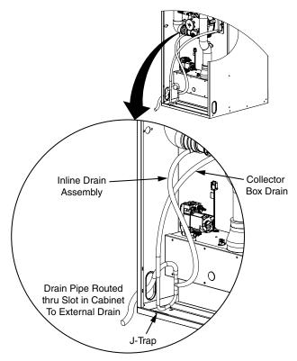
Figure 17. Condensate Drainage
