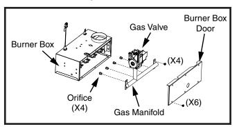
Figure 20. Orifice Removal
