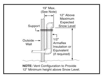
Figure 3. Alternate Horizontal Vent Installation
