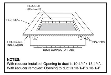
Figure 8. Duct Connector
