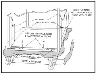
Figure 16. Cabinet Furnace on Supply Air Duct
