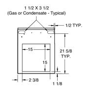
Figure 24. Front Return Cabinets (Without Coil Box)
