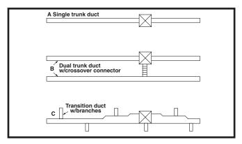
Figure 6. Typical Supply Duct Systems
