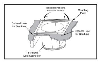
Figure 15. Round Duct Connector
