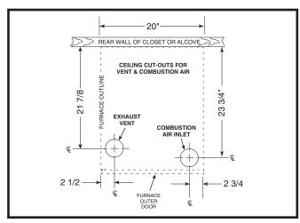
Figure 10. Ceiling Cut-Out Dimensions
