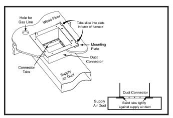
Figure 11. Finger Tabbed Duct Connector
