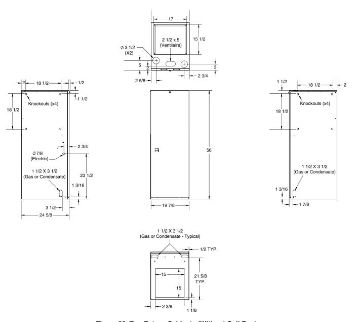
Figure 26. Top Return Cabinets (Without Coil Box)
