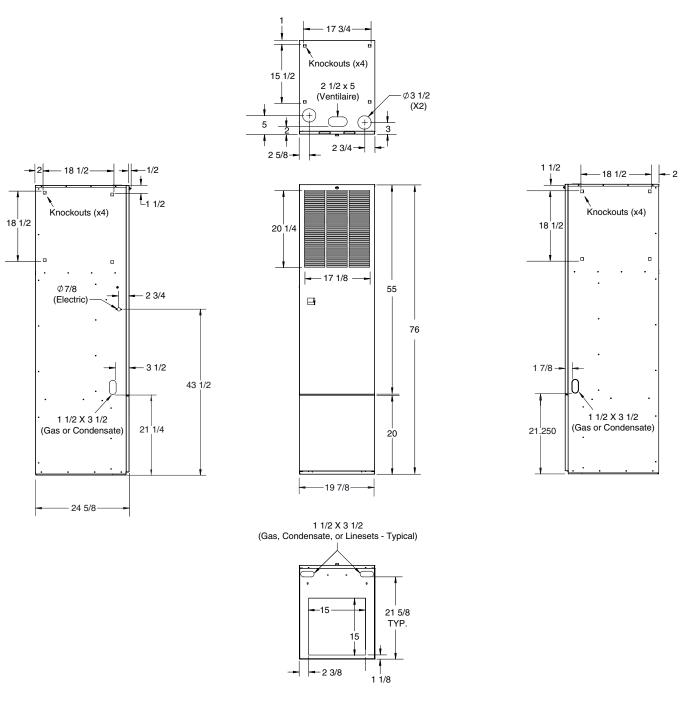
Figure 25. Front Return Cabinets (With Coil Box)
