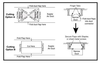
Figure 12. Screw-Down Duct Connector
