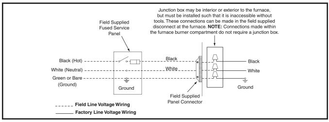
Figure 21. Line Voltage Field Wiring
