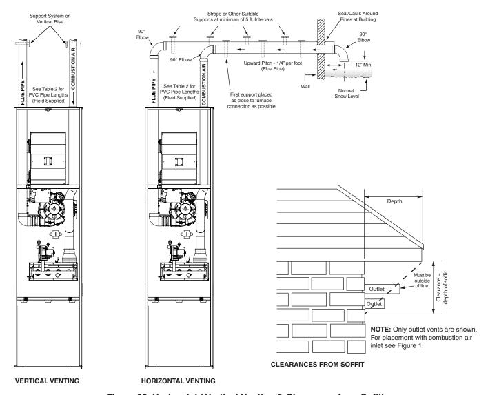
Figure 30. Horizontal / Vertical Venting & Clearances from Soffit
