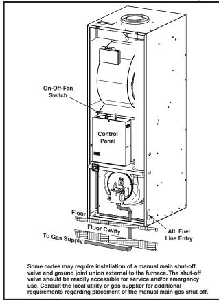
Figure 26. Typical Gas Piping
