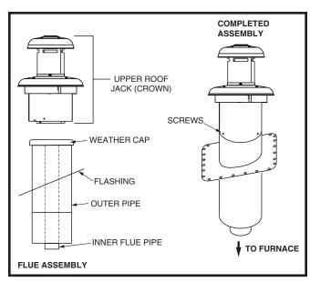
Figure 23. Roof Jack Crown
