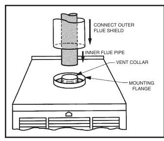
Figure 22. Combustion Air Pipe Connection
