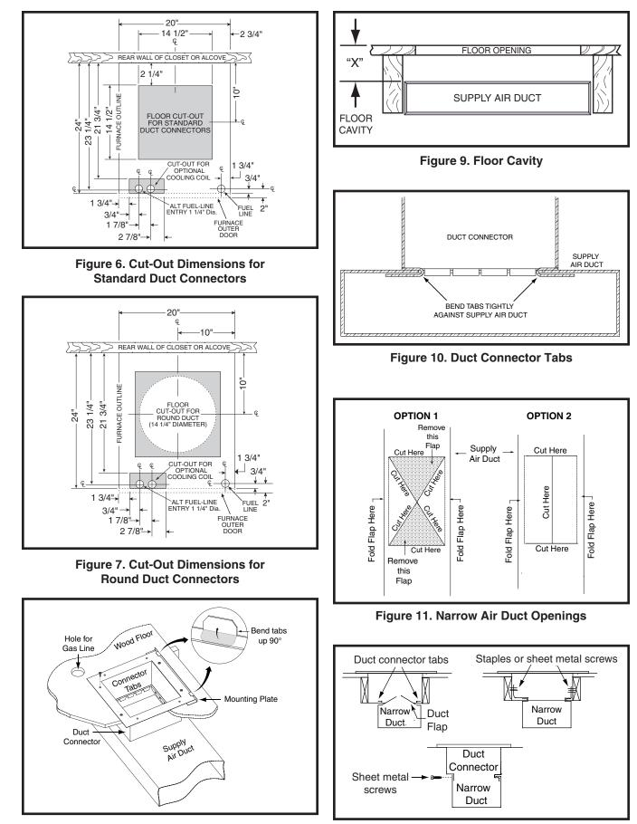
Figure 8. Standard Duct Connector Installed
