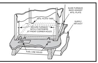
Figure 15. "A" Cabinet Furnace on Coil Cabinet
