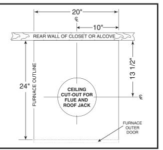
Figure 19. Cut-Out Dimensions for Flue & Roof Jack
