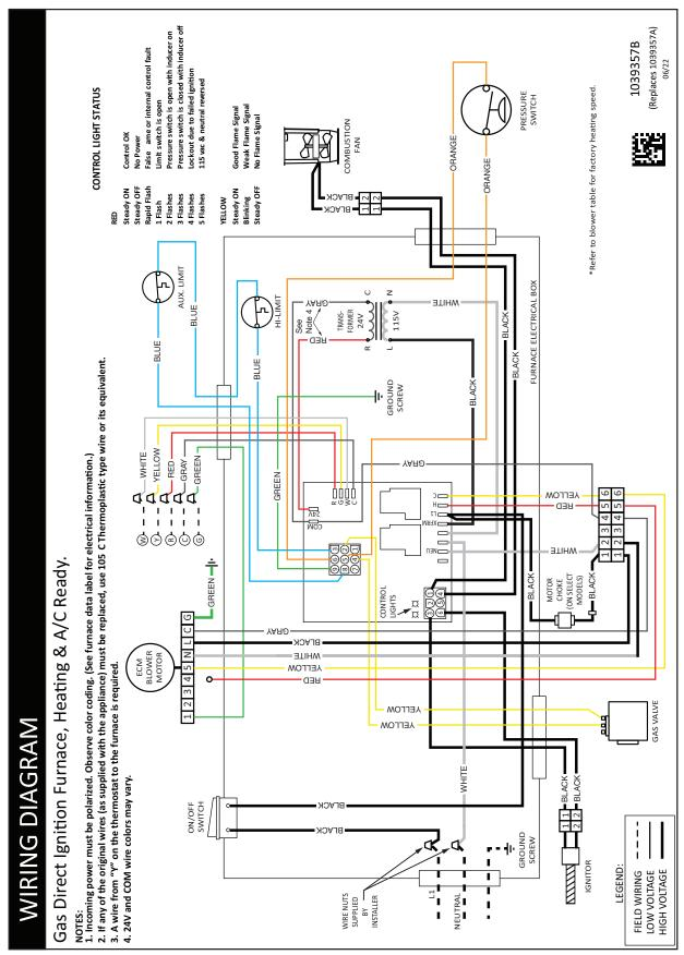
Figure 31. Gas Direct Ignition Furnace, Heating & A/C Ready - All MG1 Models
