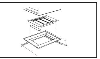
Figure 30. Without Coil Cavity Damper
