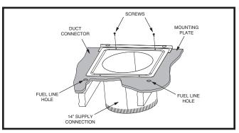
Figure 13. Round Duct Connector Installed
