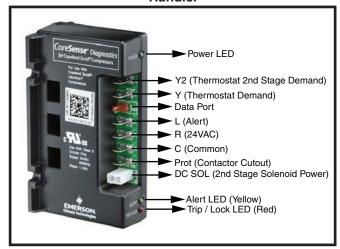
Figure 3. CoreSense™ Diagnostics Module
