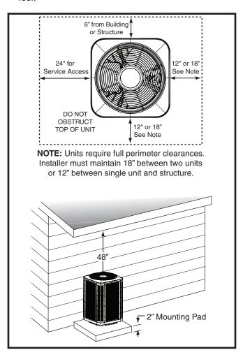
Figure 1. Clearance Requirements
