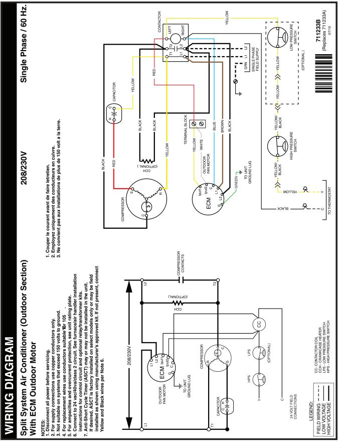
Figure 6. Wiring Diagram for \*SA(1,2)BF4M1SN (4 Ton Units)
