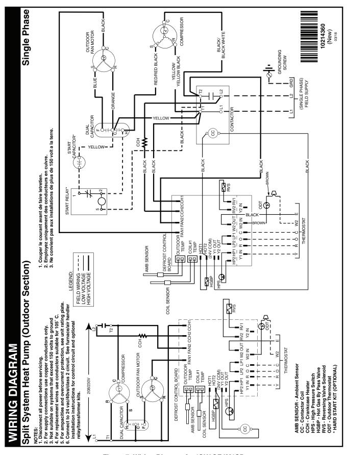
Figure 7. Wiring Diagram for \*SH2QE4M1SP
