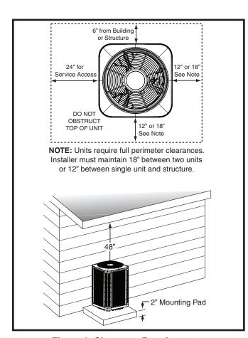
Figure 1. Clearance Requirements
