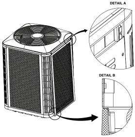
Figure 4. Panel Installation
