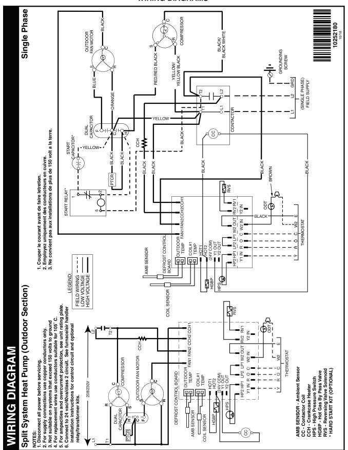
Figure 6. Wiring Diagram for \*SH2QE4M1RP
