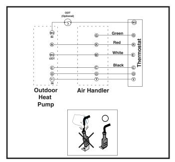
Figure 2. Typical Thermostat Connections
