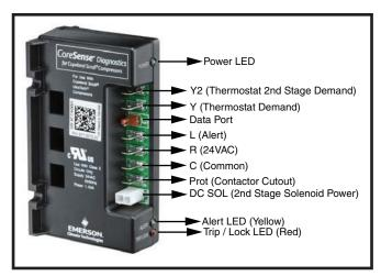
Figure 2. CoreSense™ Diagnostics Module
