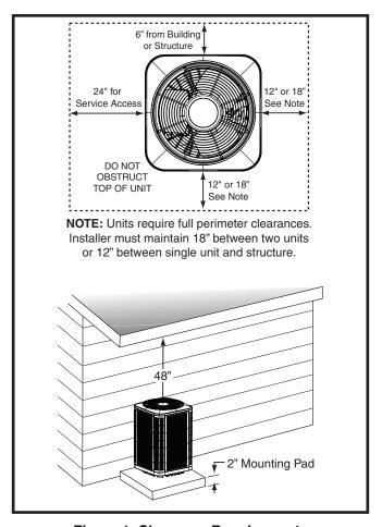
Figure 1. Clearance Requirements
