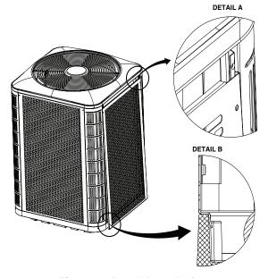
Figure 5. Panel Installation
