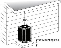
Figure 1. Clearance Requirements
