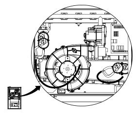
Figure 12. Pressure Switch Tubing for \*TE Upflow Furnaces
