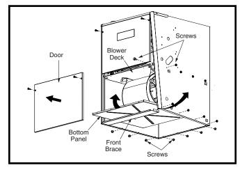
Figure 17. Alternate Removal Method
