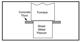
Figure 11. Furnace on a Concrete Slab
