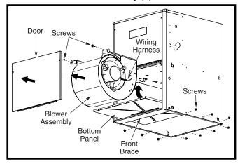
Figure 16. Bottom Panel Removal
