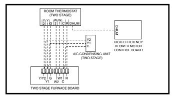
Figure 22. Wiring Configuration 3
