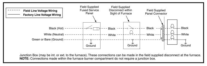
Figure 19. Line Voltage Field Wiring
