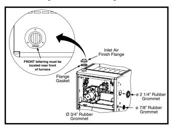
Figure 14. Finish Flange & Rubber Grommets
