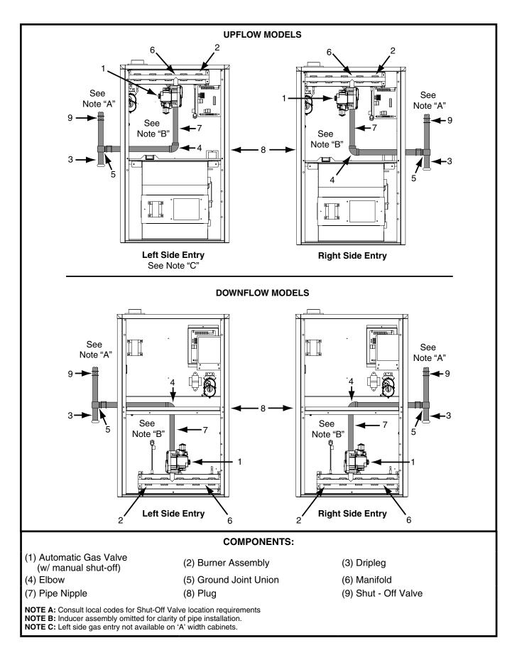
Figure 18. Typical Gas Connections
