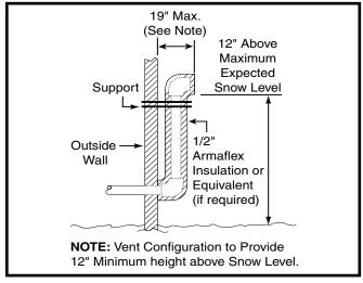
Figure 9. Alternate Horizontal Vent Installation
