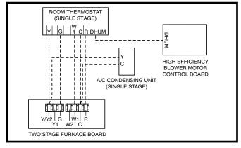
Figure 20. Wiring Configuration 1
