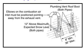
Figure 10. Vertical Vent Termination
