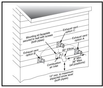
Figure 7. Inlet & Exhaust Pipe Clearances
