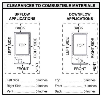
†Allow 24 in. minimum clearance for servicing. Recommended clearance is 36 in.
