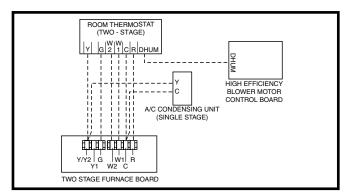
Figure 21. Wiring Configuration 2
