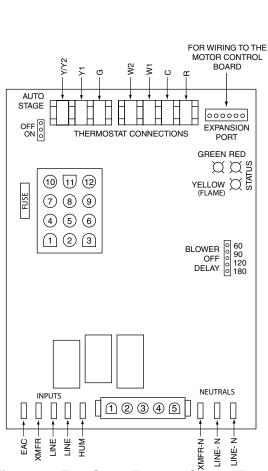
Figure 29. Two-Stage Furnace Control Board
