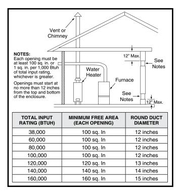
Figure 2. Combustion Air Drawn from Inside
