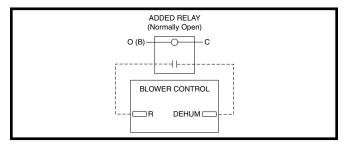
Figure 24. DEHUM Wiring Configuration without Humidistat
