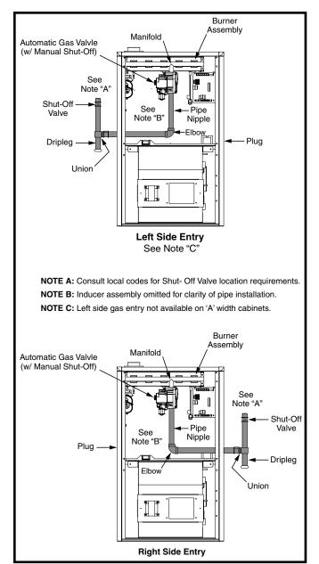
Figure 18. Typical Gas Connections
