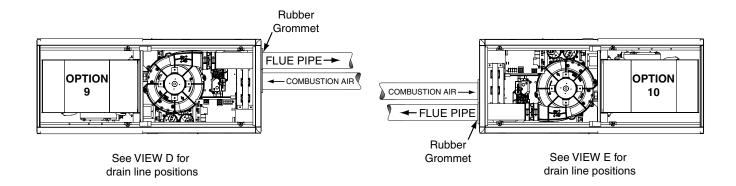
Figure 36. Horizontal Venting Options (A Width Cabinets)
