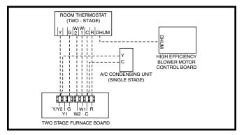
Figure 21. Wiring Configuration 2
