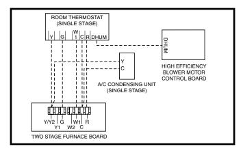
Figure 20. Wiring Configuration 1
