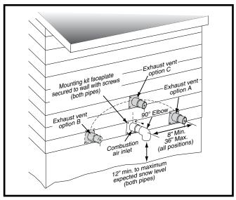
Figure 7. Inlet & Exhaust Pipe Clearances
