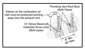
**Figure 10. Vertical Vent Termination**
