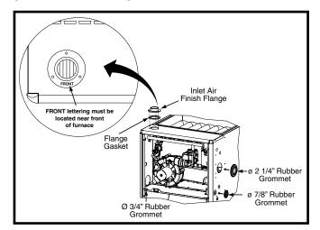
Figure 14. Finish Flange & Rubber Grommets
