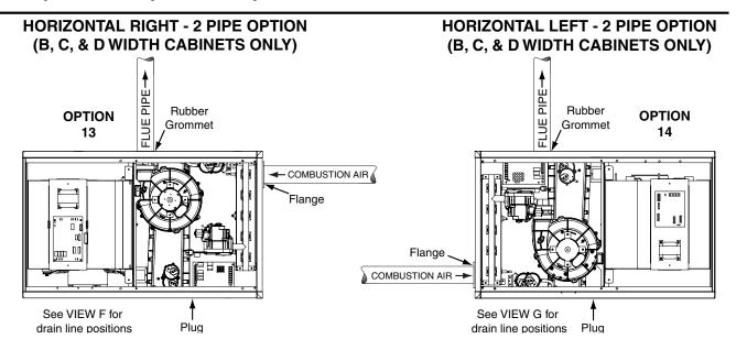
Figure 37. Horizontal Venting Options (B, C, & D Width Cabinets)
