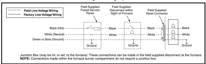
Figure 19. Line Voltage Field Wiring
