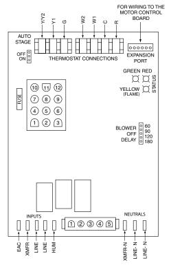
Figure 29. Two-Stage Furnace Control Board
