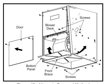
Figure 17. Alternate Removal Method
