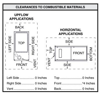
$\uparrow$ Allow 24 in. minimum clearance for servicing. Recommended clearance is 36 in.
