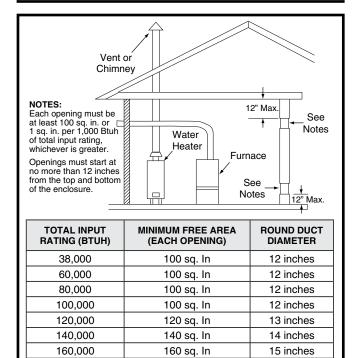
Figure 2. Combustion Air Drawn from Inside
