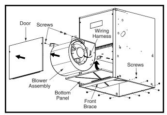
Figure 16. Bottom Panel Removal
