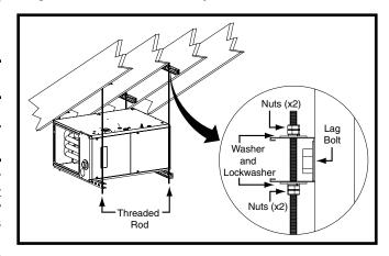
Figure 12. \*TC Horizontally Suspended in Attic
