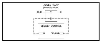
Figure 24. DEHUM Wiring Configuration without Humidistat
