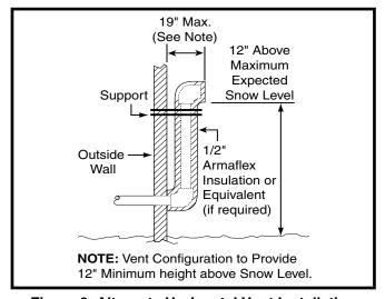
Figure 9. Alternate Horizontal Vent Installation
