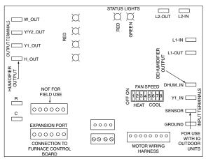
Figure 28. Two-Stage Variable Speed Motor Control Board
