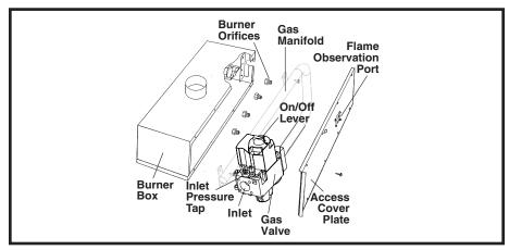
Figure 2. Typical Sealed Burner Box With Access Cover Plate
