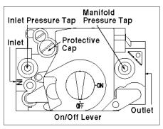
Figure 4. Gas Valve (Honeywell shown)
