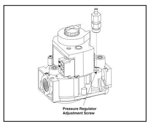
Figure 3. Pressure Regulator Adjustment Screw Location (VR8205S 2288)
