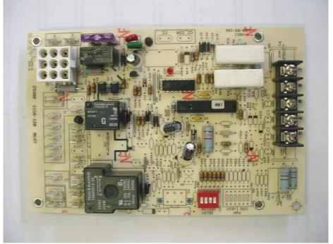
FIGURE 5: UNITED TECHNOLOGIES 1168-1 ECM TAP BOARD (O4HD-091A-V-FA)
