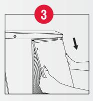
To reinstall, repeat these steps in reverse, making sure to seat the bottom of the panel on the lip of the base pan.
