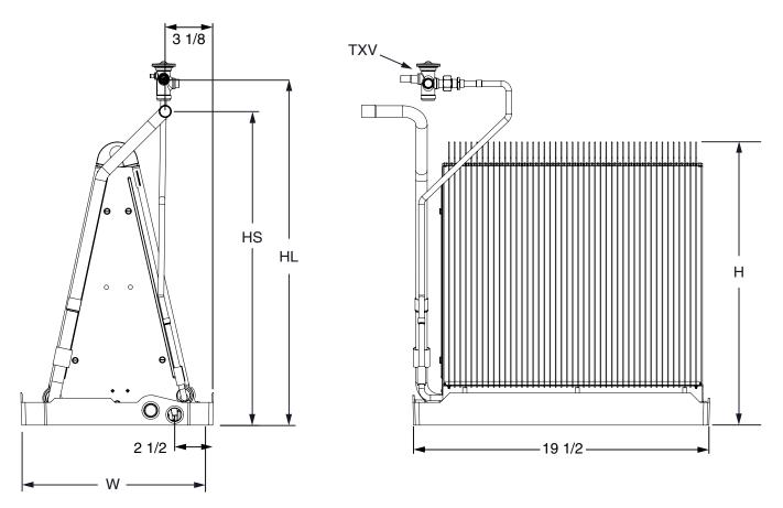
Figure 1. C7 Coil Dimensions (with TXV)
