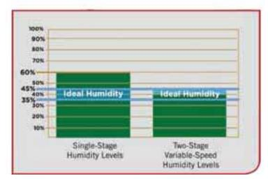
This reduced capacity is enough to efficiently cool your home on mild summer days. When the temperature rises the air conditioner or heat pump automatically adjusts itself and enters the second stage to meet the increased cooling demand.
