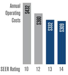
Annual costs based on 36,000 Btu unit, 1,500 cooling load hours and .08/kwh. Actual costs may vary depending on climate conditions, energy rates and patterns of usage.
