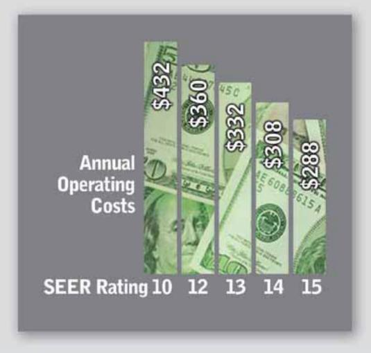
Annual costs based on 36,000 Btu unit, 1500 cooling load hours, and .08/kwh. Actual costs may vary depending on climate conditions, energy rates and patterns of usage.
