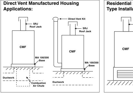
NOTE: Direct Vent Kit may be installed on either the right or left side of the furnace. \* For Non-Manufactured Housing Applications Only.
