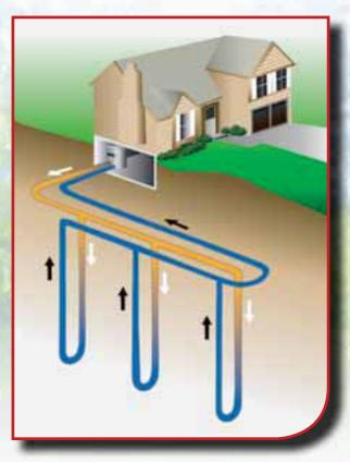
Geothermal heat pump systems consist of basically four parts: the ground heat exchanger, the heat pump unit, the indoor air handler, and the air delivery system (ductwork). The heat exchanger is basically a system of pipes called a loop, which is buried in the shallow ground near the building. A fluid (usually water or a mixture of water and antifreeze) circulates through the pipes to absorb or relinquish heat within the ground.
