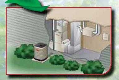
iQ Drive heat pump systems consist of basically four parts: the outdoor heat pump, the indoor air handler or furnace with coil, an iQ Drive thermostat, and the air delivery system (ductwork).
