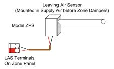
NOTE: If the PCZPS is not used, the NO SENSOR jumper located just above the LAT terminals must be on the pins.
