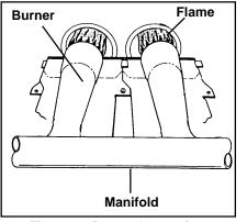
Figure 2. Burner Inspection
