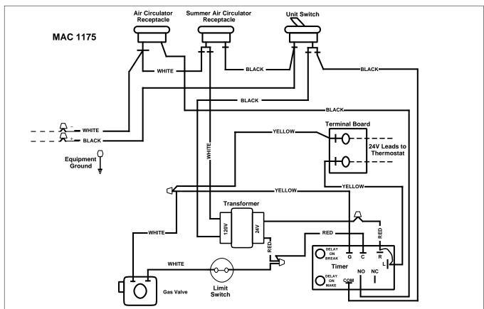
Figure 1. MAC 1175 Wiring Diagram
