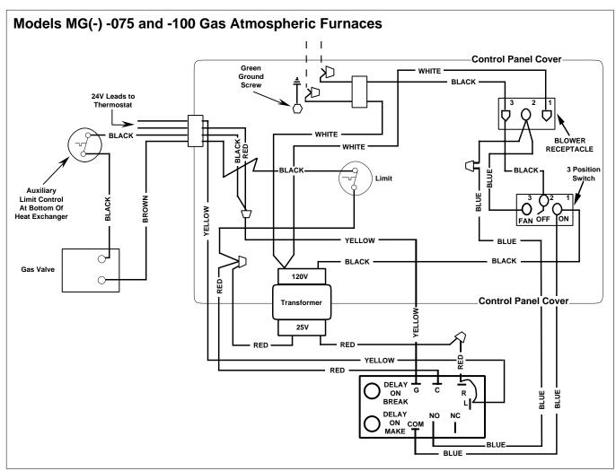
Figure 2. MGH Furnace Wiring Diagram
