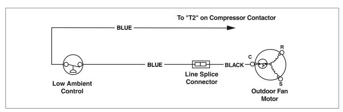
Figure 1. Air Conditioner Low Ambient Control Kit Wiring Diagram
