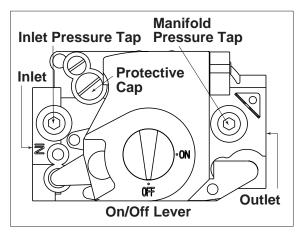
Figure 4. Gas Valve (Honeywell shown)
