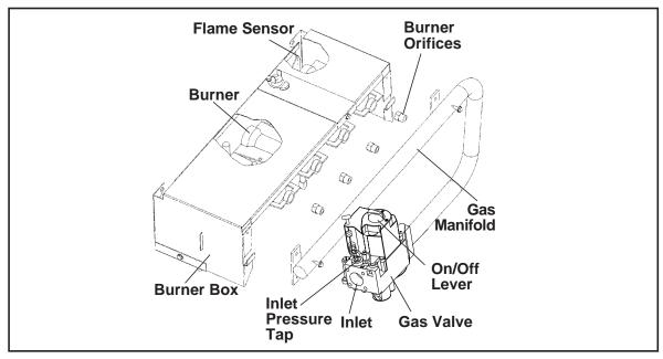
Figure 1. Typical Non-Sealed Burner Box
