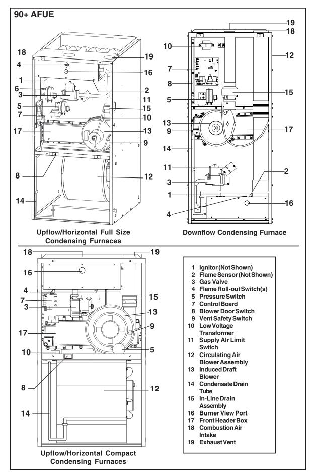
Figure 2. Furnace Parts Identified
