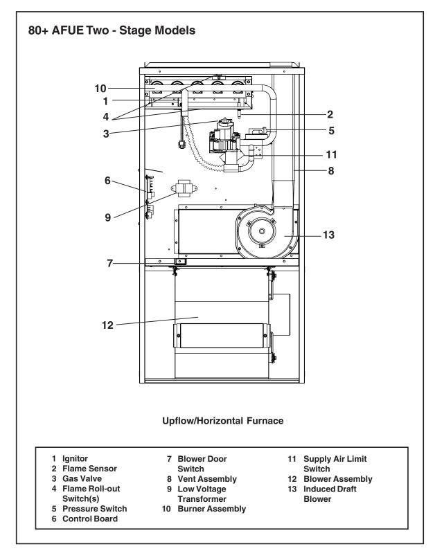
Figure 4. Furnace Parts Identified
