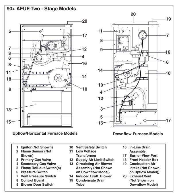
Figure 3. Furnace Parts Identified
