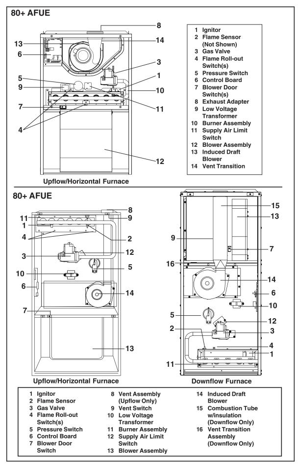
Figure 1. Furnace Parts Identified
