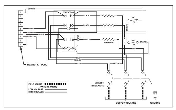
Figure 7. Typical 3-Phase System Wiring Diagram
