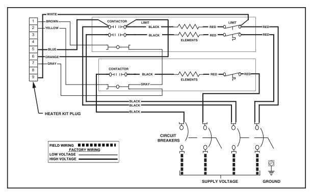
Figure 6. Typical System Wiring Diagram
