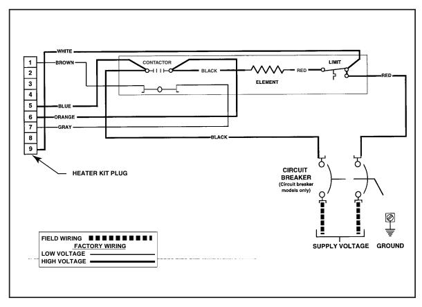
Figure 4. Typical System Wiring Diagram 5 kw 1-stage with circuit breaker
