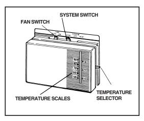
Figure 1. Typical Thermostat
