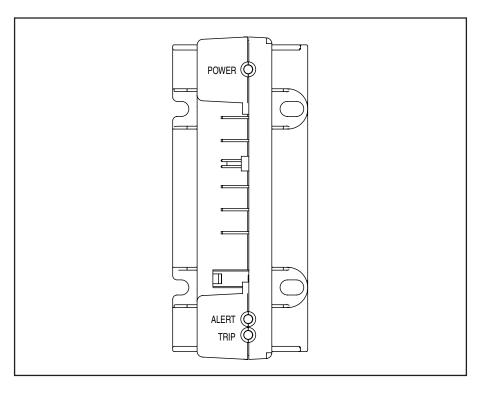
Figure 2. Comfort Alert™ Diagnostics Module
