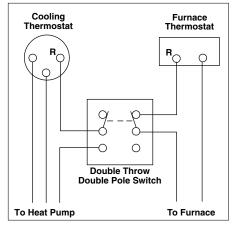
Figure 2. Thermostat Interlock System
