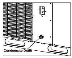
Figure 5. Condensate Drain
