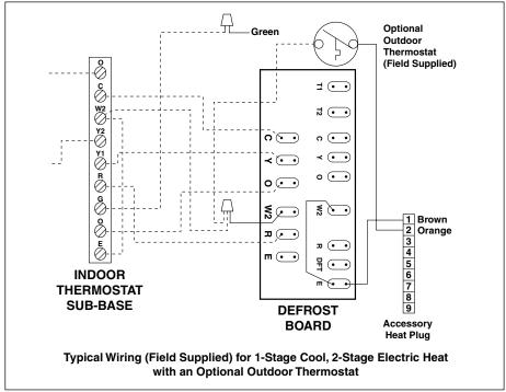
Figure 8. Typical Heat Pump Thermostat Connections
