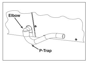
Figure 6. Drain Trap
