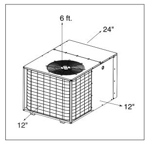
Figure 2. Minimum Unit Clearances
