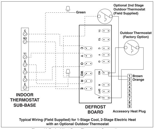
Figure 10. Typical Heat Pump Thermostat Connections
