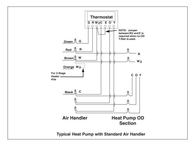
A typical installation with a heat pump thermostat, air handler, and heat pump with an outdoor thermostat.
