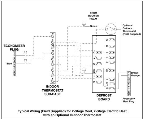
Figure 10. Typical Heat Pump Thermostat Connections
