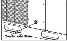
Figure 5. Condensate Drain
