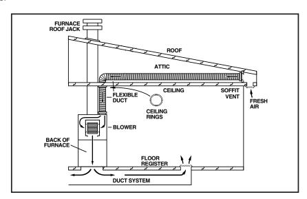
Figure 5. General Install Setup
