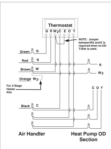
**Typical Heat Pump with Standard Air Handler**
